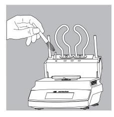
3) Clean the heating element and temperature sensor with a weak solvent such as ethanol.
